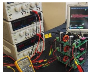
Three boost converters sharing common output power line
